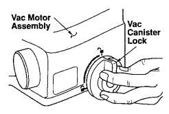
3. Place vac motor assembly onto vac canister assembly.
